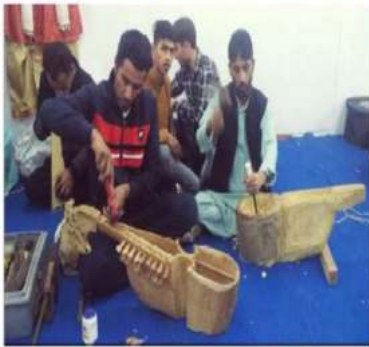
Making process of Rabab from initial to final stage (Chiseling & other wooden work)
